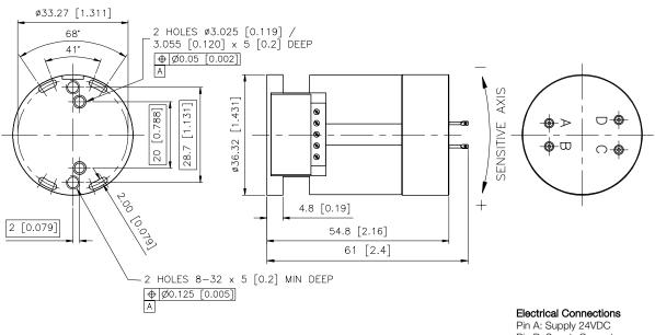
Pin B: Supply Ground Pin C: Signal Ground Pin D: Signal Output
