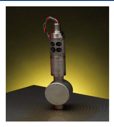
Viatran's Model 544 is a gage pressure transmitter designed for precise measurement in harsh environments. Its all welded 316 stainless steel construction ensures durability and corrosion resistance, and it offers overpressure protection to 500 PSI.
